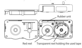
Turn the transparent reel in the OPEN direction in order to unlock while pressing the sawtoothed parts of the red reel with one hand, and pull out it.
