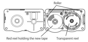
NOTE: Turn the lever a few times to remove the slack on the tape.
